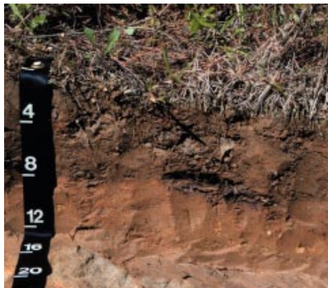
Figure 15.—Typical pedon of Wilkes sandy loam. The Wilkes soils have soft bedrock at a depth of 10 to 20 inches. Depth is marked in inches.
