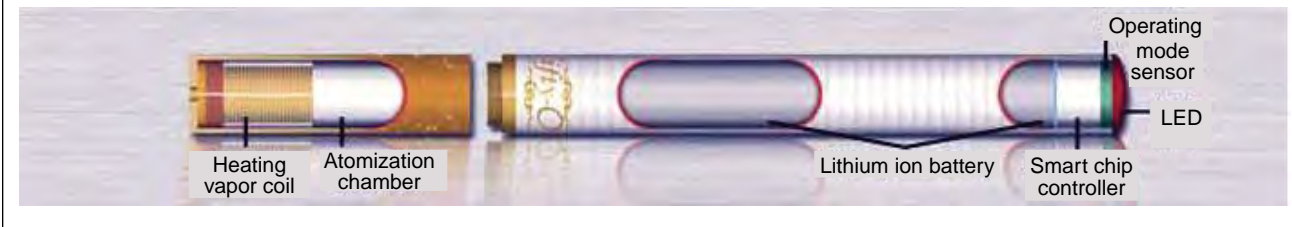
Figure 1. Basic design of an electronic cigarette.
